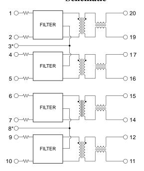
\*Note: Attach pins 3 and 8 to ground for improved common mode performance.
